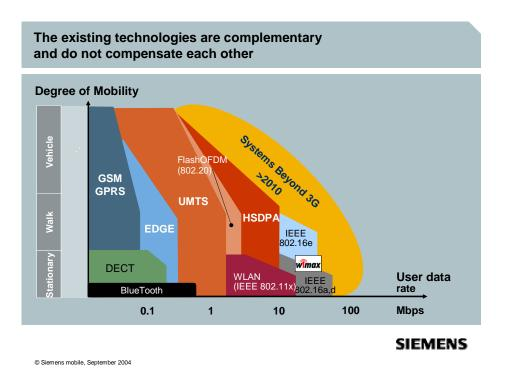
Figure: Comparing degree of mobility versus user data rate of various radio standards
